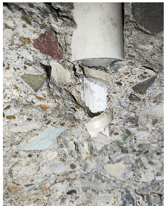
Fig. 14. Cross-section of the failure location.
